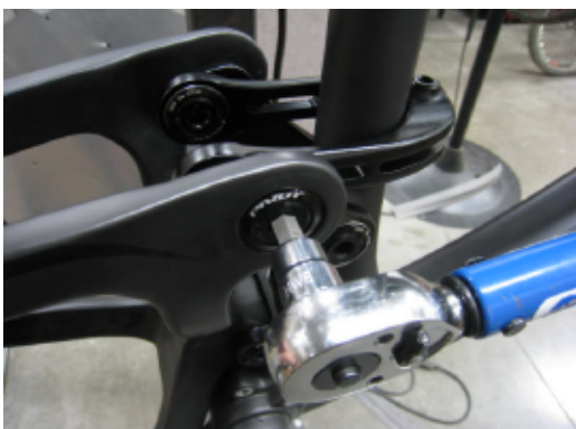
50 Torque bolts to 35Nm
