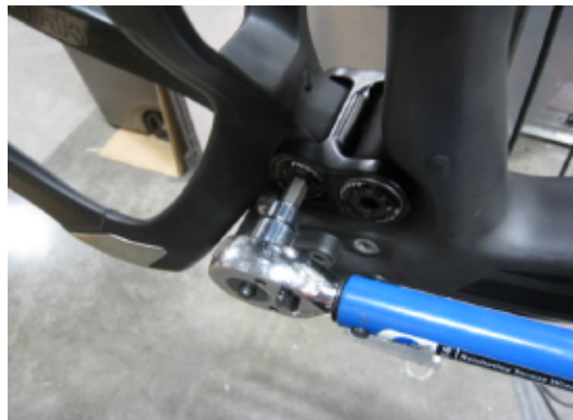
47 Torque bolts to 35Nm
